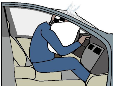
Movement without seat belt fastened
